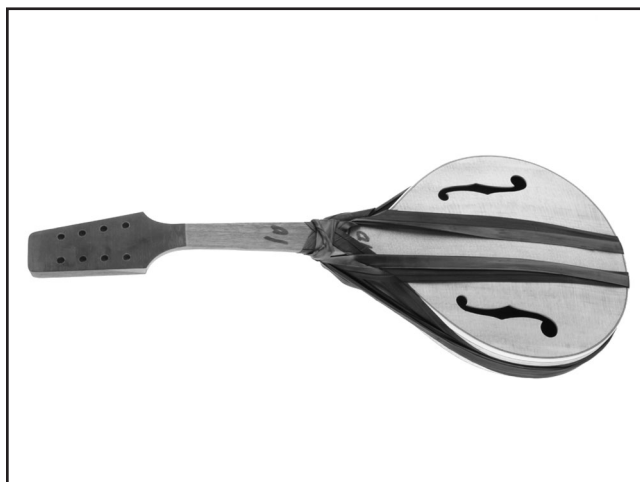
Figure 13. Example of gluing the neck.
